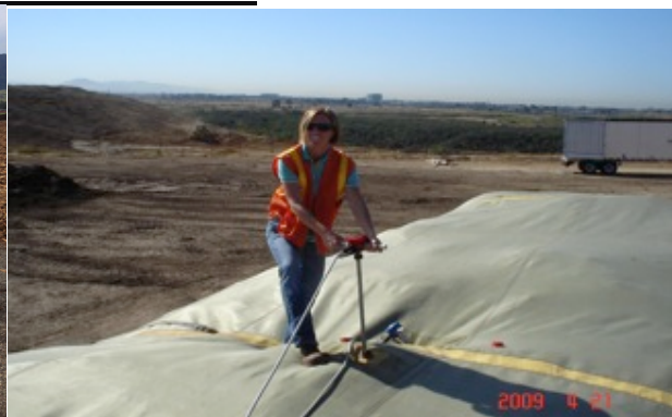
LOWER RIGHT: Technician inserting probes into pile through the GORE® Cover
