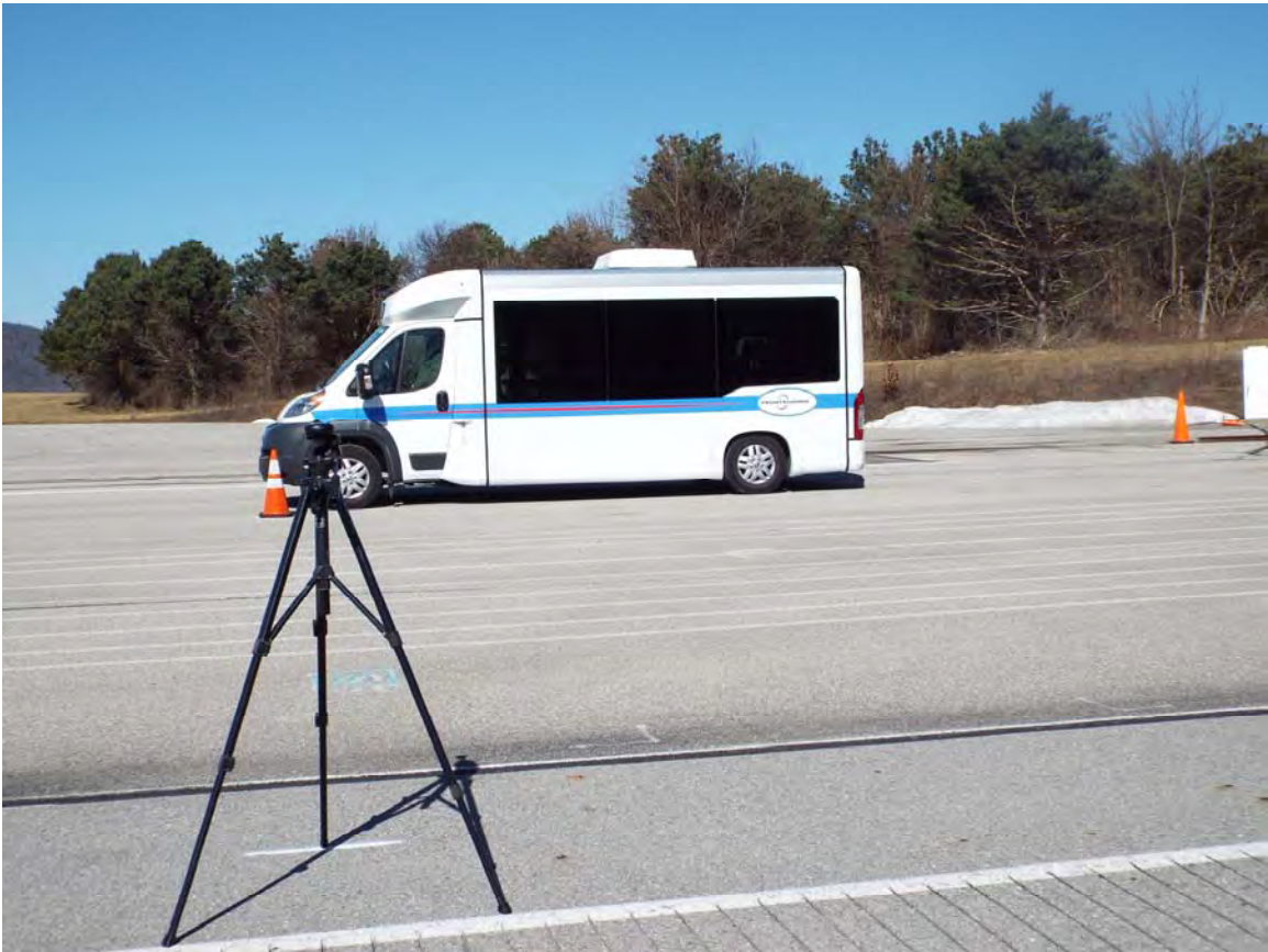
TEST BUS UNDERGOING EXTERIOR NOISE TESTING
