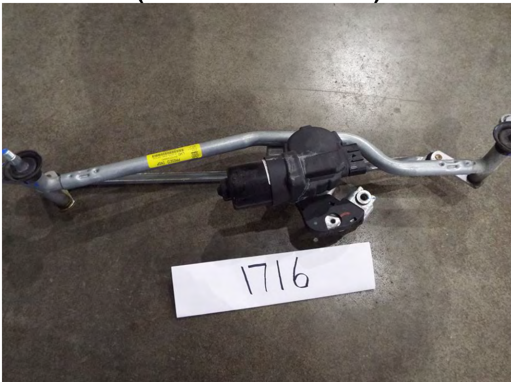
WIPER MOTOR REMOVAL AND REPLACEMENT (0.75 LABOR HOURS)
