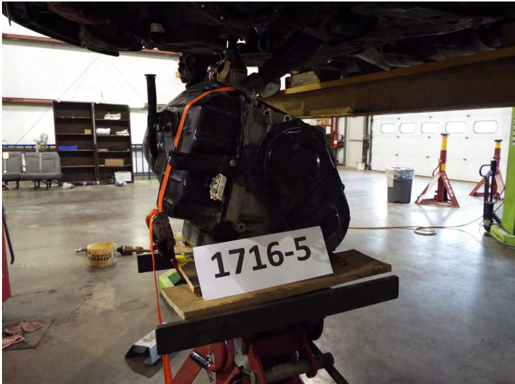
TRANSMISSION REMOVAL AND REPLACEMENT (8.50 LABOR HOURS)
